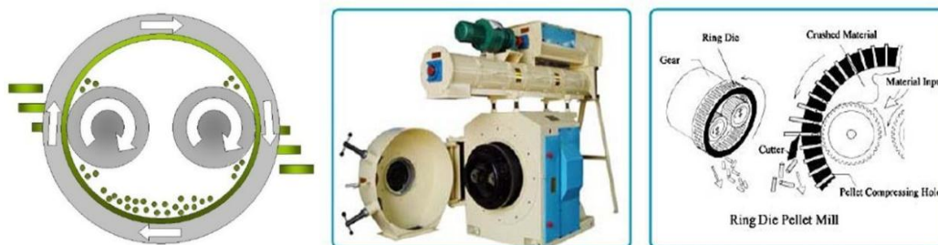
Figure 3. The working principle of pellet machine with ring matrix
