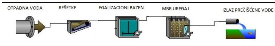
Figure 2. Sewage treatment plant using MBR device
