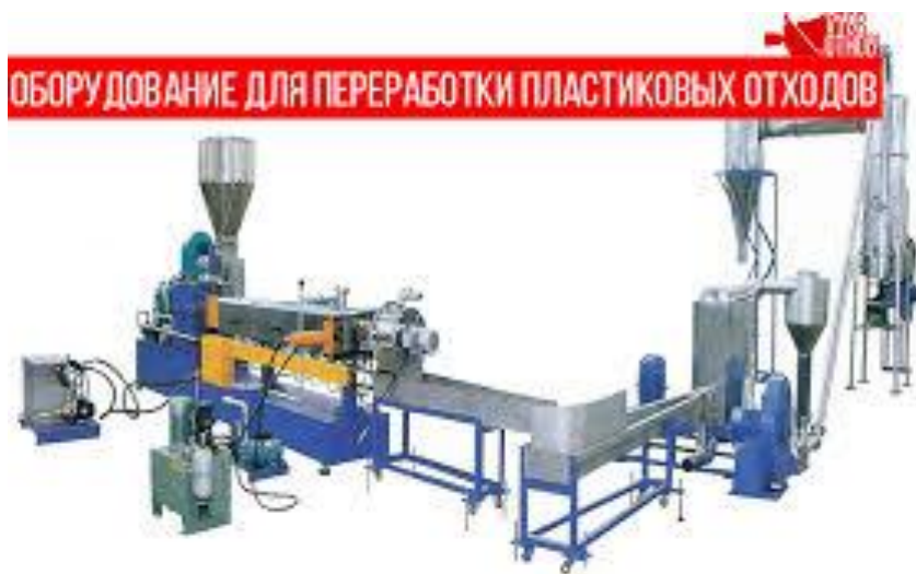
Fig. 2: Line for processing in-dustrial and ho-usehold waste from plastic
