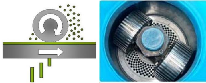
Figure 2. The working principle of pellets machine with a flat matrix
